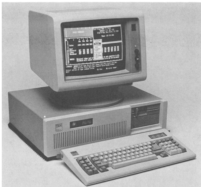
FIG. 1—IBM-PC-AT Supermicro computer with monitor screen, 20-megabyte hard disk, floppy disk drive, and keyboard (Compliments of International Business Machines, Inc.).
