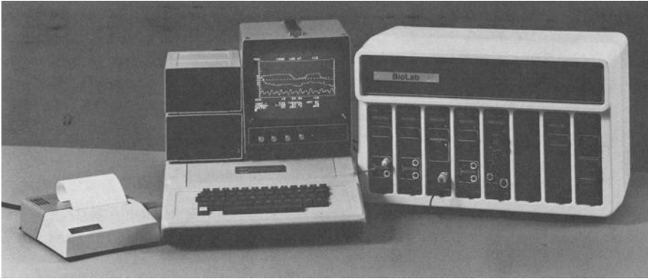
FIG. 4— Bilog System. Left to right: thermal printer, two floppy disk drives, Apple II computer, monitor, amplifier, analog to digital (A/D) circuit system for lab equipment (Compliments of Cyborg, Inc.).
